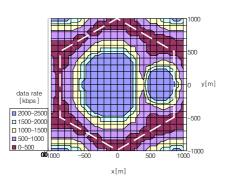
Fig. 5. The distribution of data rate in the hierarchical highspeed data system.
