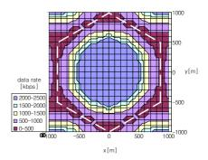
Fig. 3. The distribution of data rate for high-speed data system.
