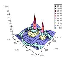
Fig. 4. The C/I distribution in the hierarchical high-speed data system.
