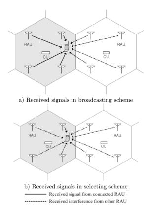
Fig. 1. Transmission schemes in bunched system
