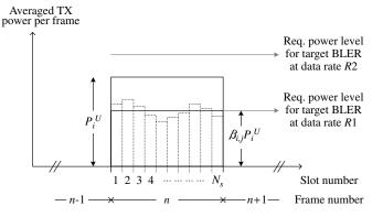
Fig. 1. Example of the power and rate assignment.
