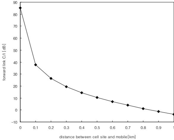
Fig. 2. The C/I of the high-speed data system Forward link, the Tx power of AP = 20W.
