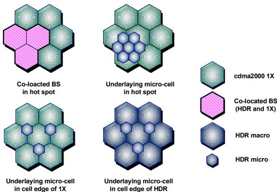
Fig. 1. Cell deployment strategies of the high-speed data systems.
