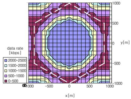
Fig. 3. The distribution of data rate for high-speed data system.
