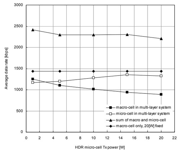
Fig. 7. The average data rate of macro/micro-cell cell with various Tx power of micro-cell.
