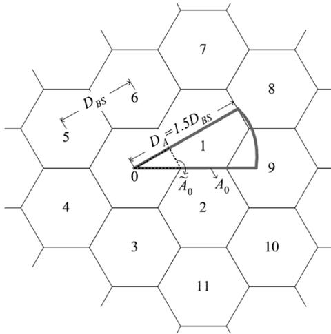
Fig. 1. Cell site deployment model.
