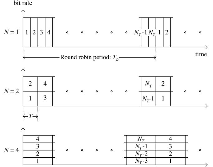
Fig. 2. Example of packet transmission with various numbers of simultaneous users.
