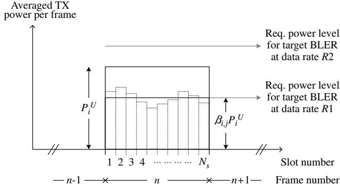
Fig. 1. Example of the power and rate assignment.
