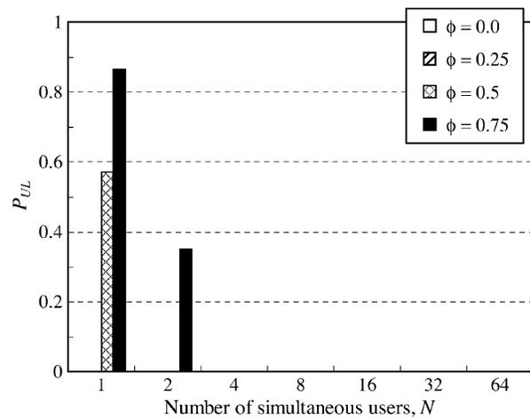
Fig. 6. Probability of the assigned data rate being limited by the data rate set.
