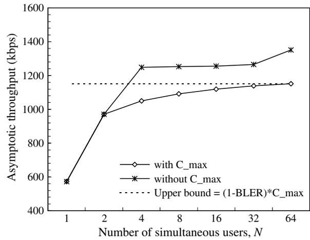
Fig. 10. Effect of code shortage on the system throughput:  $\phi = 0.75$ .
